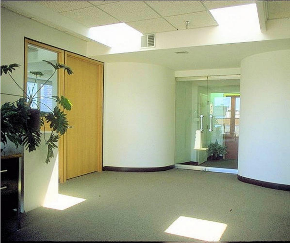
Effective daylighting designs do much more than just let in more light through the window. Indeed, direct beam sunlight through windows and skylights (like the case illustrated) can produce very bright areas that can make the lighting environment quite uncomfortable.
