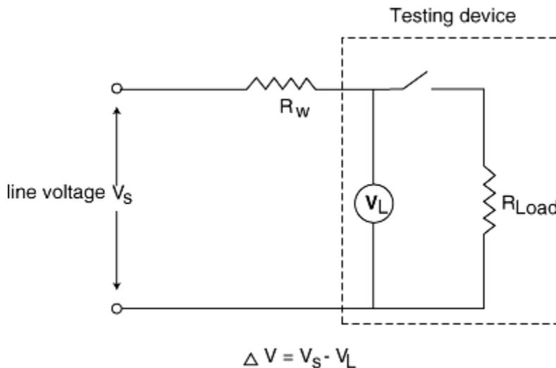
**Figure 1.** Schematic of a branch circuit wiring analyzer.
