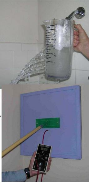
well. Ducts that show the greatest pressure readings are usually closest to the leaks, a powerful aid in the sealing process the audit will recommend.
