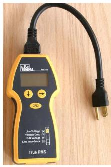
The auditor routinely checks for gas leaks (using an electronic **sniffer** like the one shown) as well as for poor or corroded electrical wiring connections between the circuit breaker box and outlets. The **circuit tester** pictured works like a stress-test EKG by putting a 15 amp load on a circuit for a few milliseconds while measuring the voltage drop due to the load. A five percent or more drop suggests the need for remediation.
