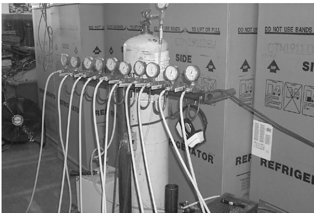
4. Refrigerant extractor (does 10 at a time in about 12 minutes)
