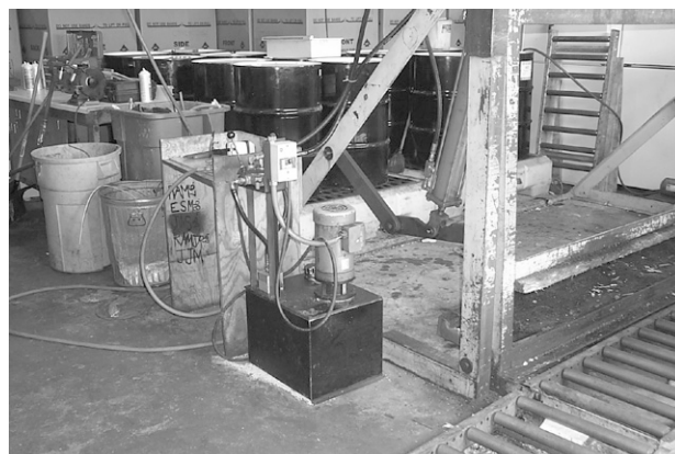
8. Hydraulic system for tipping refrigerators to drain oil
