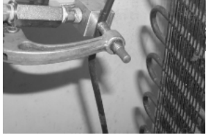
3. First step: refrigerant extraction
