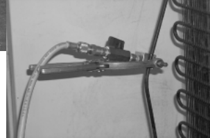
3. First step: refrigerant extraction
