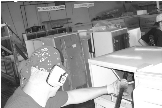
13. A mining bar employed with a delicate touch separates plastic and aluminum from steel
