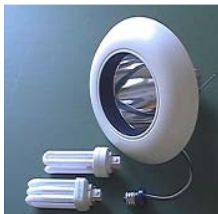
Figure 10. The PowerLux system keeps the ballast outside of the can. Replaceable CFLs that fit the system are available in 18, 26, 32, and 42 watts, and in color temperatures of 2700, 3000, 3500 or 4100K.
