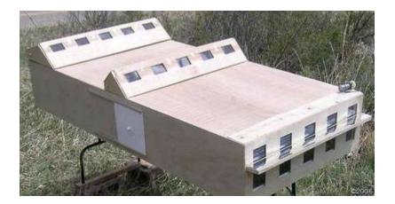
**\*Smart Light Shelves**, sidelighting systems which are manipulated to optimize the distribution of light as deeply as possible within a structure while constraining direct beam sunlight from falling on work spaces.
