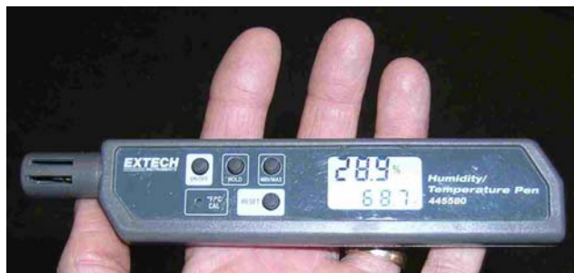
Figure 1. This humidity/temperature sensor fits in a shirt pocket.
