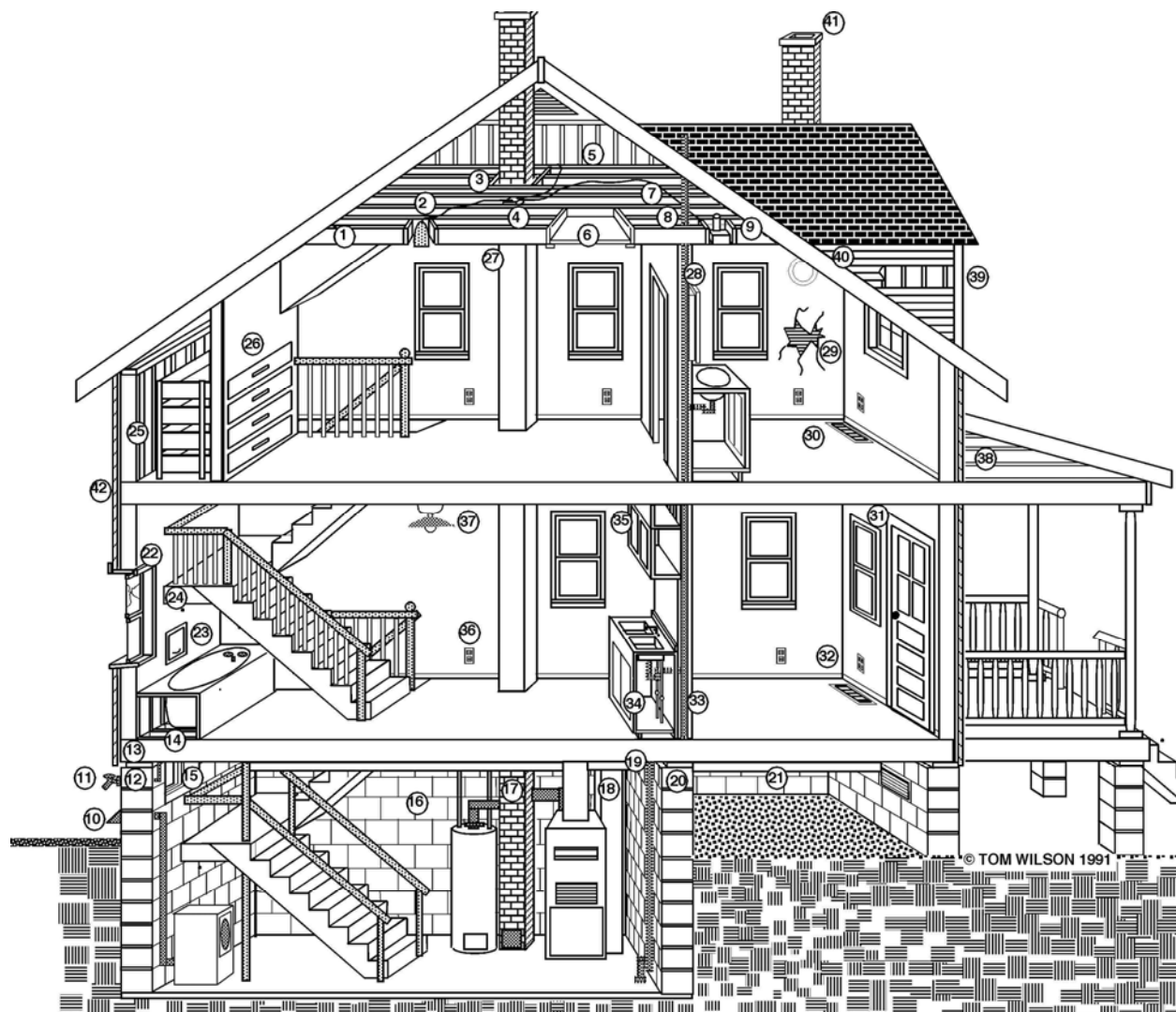
Figure 8. Some areas where air infiltration/exfiltration may occur in a dwelling.
