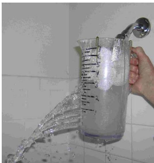
Figure 25. Measuring shower flow rate using a weir avoids needing a stop watch. Just wait until the water comes to the highest hole and read the flow rate on the side of the weir. The procedure only takes 15 seconds or so.
