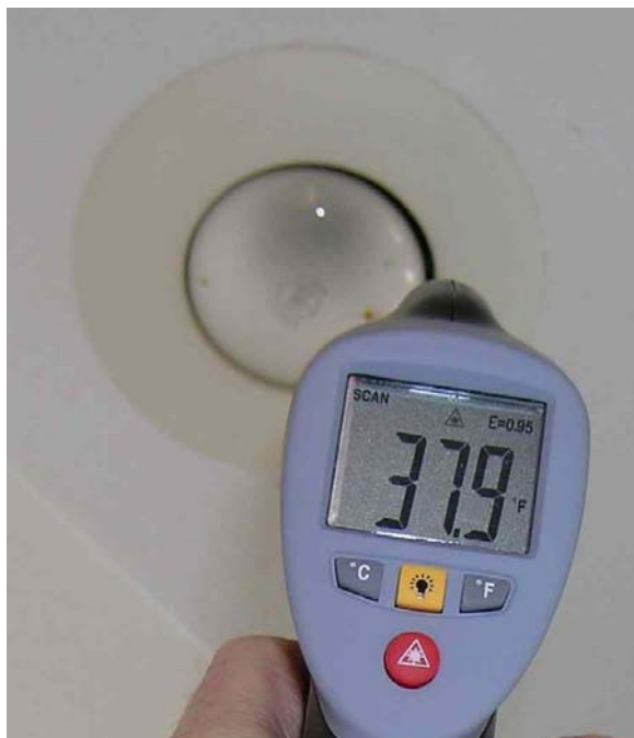
Figure 31. Kitchen light in a home heated to 68°F, outside air temperature of 34°F, blower door depressurizing the home drawing in the cold attic air.
