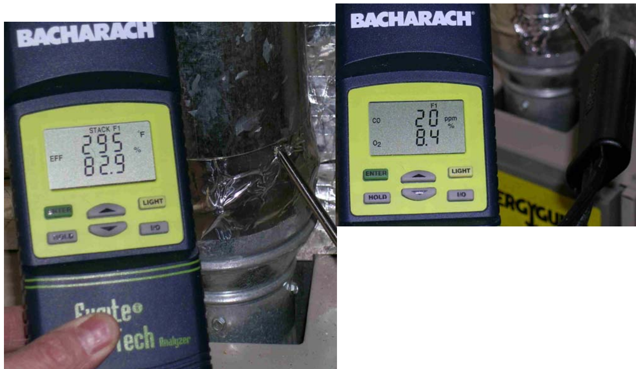
Figure 19. Bacharach furnace tester measuring stack temperature and % steady state efficiency (left) and parts per million of CO and % oxygen in the stack gas (right)
