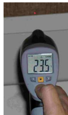
Figure 12. A cold spot near the interface of a wall and a cathedral ceiling containing 10 inch batts of fiberglass indicates an area of air infiltration. Picture taken when outside temp was 10F and inside temp 65F; the area surveyed is at 23.5F.
