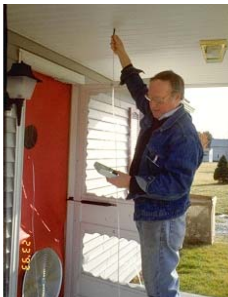
Figure 10. Substantial pressure readings suggest that a porch may be effectively within the conditioned envelope.
