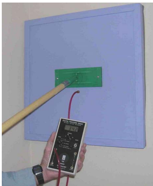
Figure 13. Duct pan over large return indicates substantial leakage, 34 pascals
