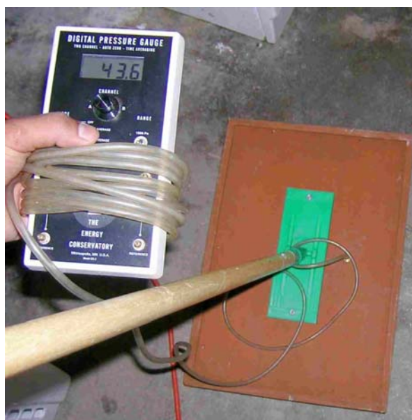
Figure 14. Smaller duct pan for supply ducts can also be used for taking other pressure measurements, in this case a drain in the basement floor suspected of a leaky trap.
