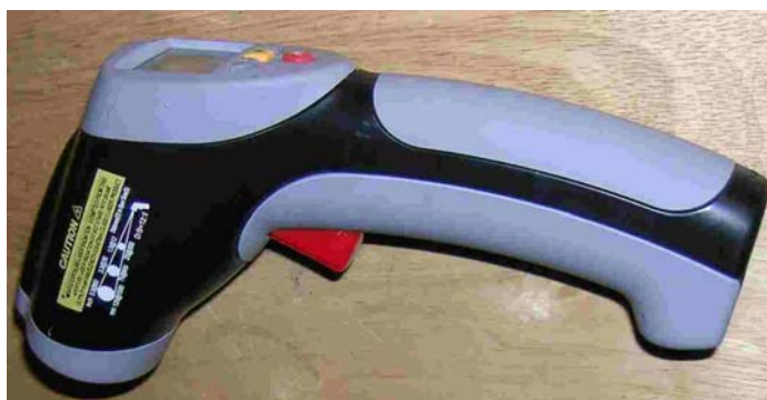
Figure 11. This spot radiometer takes temperatures at a distance. A laser that is bore sighted with the center of the field of view of the instrument may be turned on to indicate precisely where surface temperatures are sampled.
