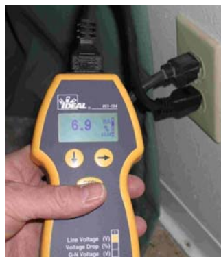
Figure 2. Ideal circuit tester. Refrigerators and freezers represent a substantial portion of the electric bill in many homes, nationally about 12%. Since many older units use 1,000 kWh/year or more—and new ENERGY STAR-rated units well less than 500 kWh/year—it is useful to measure their consumption toward estimating the cost effectiveness of replacement.
